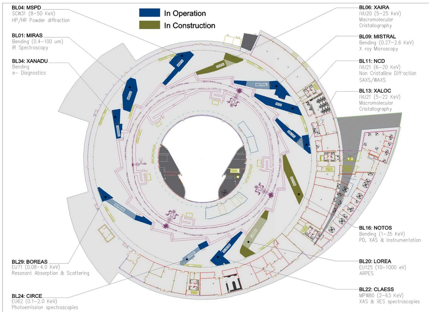
Figure 1 – ALBA Layout including beamlines and accelerators.
