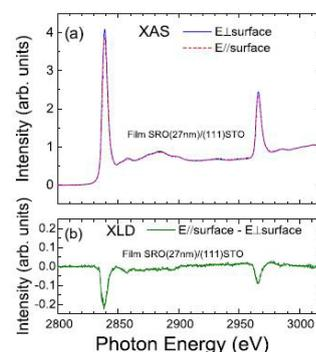
Figure 2 - a) X ray absorption spectra at the Ru  $L_3$  and  $L_2$  absorption energies from a 27 nm ferromagnetic film of  $\text{SrRuO}_3$  grown on  $\text{SrTiO}_3$ . The photon beam was linearly polarized with the polarization either parallel (red curve) or perpendicular (blue) to the film surface. b) Linear dichroism spectrum obtained subtracting the two spectra in (a).
