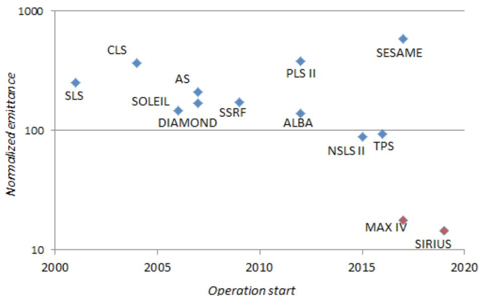
Figure 8 – Emittance normalized with circumference and square of energy plotted versus year of operation start of light sources included in Table 4. Blue dots correspond to 3rd generation light sources, red to 4th ones.
