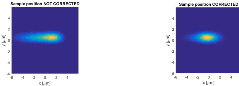
Figure 32. Beam spots at sample position including the thermal deformation of the HPM and X1, and the slope errors of the HPM, VFM and HFM. ( left ) Beam spots without refocusing the optics. ( right ) Beam spots after refocusing the VFM and/or the HFM. The variation of the focal distance \Delta q_{h,v} is listed in Table 13 for all cases.
