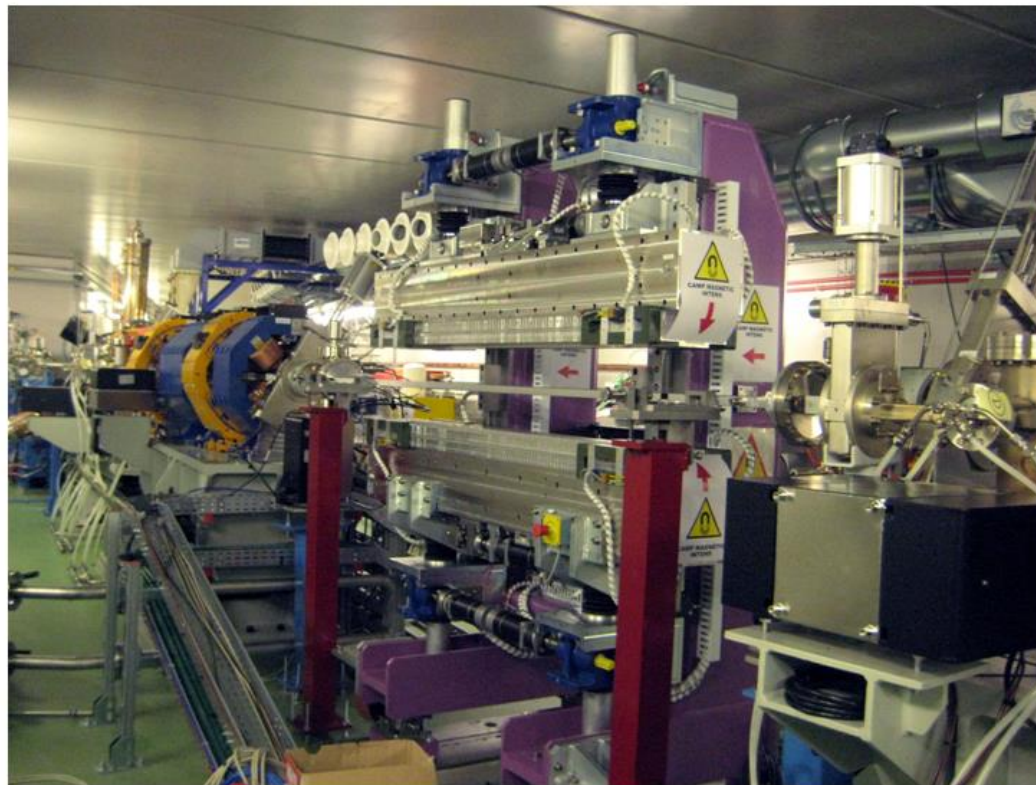
Figure 2. This picture shows the first Insertion Device installed in the ALBA Storage Ring. It is an APPLE-II Undulator, with a period of 71 mm which will give light to BL29-BOREAS.
