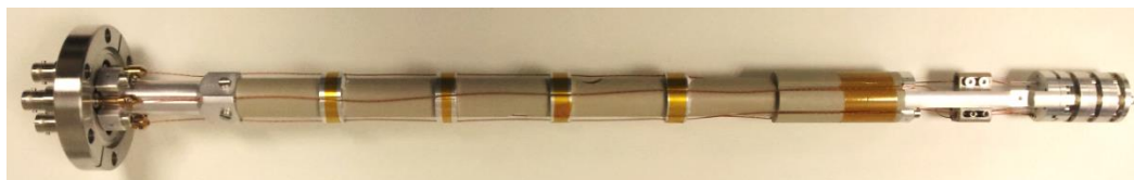
Fluorescence diode assembly designed and built at ALBA (installed end Feb'2013)
