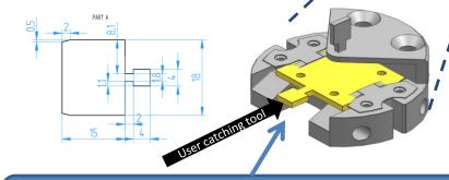
The traveler attached to the magnetic arm offers the "spoon" of the sample plate to the docked chamber allowing users to directly catch the omicron-like sample plate spoon Please remember to contact the BL staff during proposal writing if you are willing to bring your chamber to be docked to the UHV-SPTR!!
