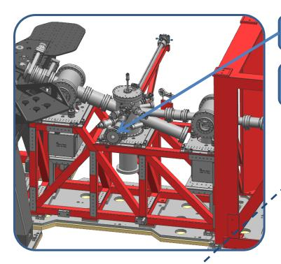
The docking port on the central distribution chamber of the UHV-SPTR system
