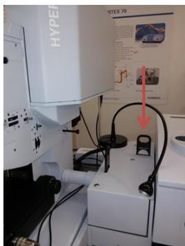
This image is showing the location of the attenuator between the microscope and spectrometer with the attenuator set.
