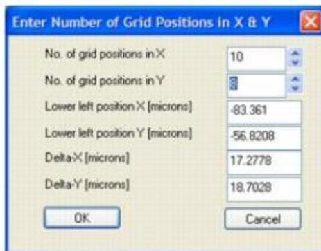
In many cases, you can increase the spatial resolution by overlapping measurement areas. For example, if you are using an aperture of  $10 \times 10 \mu\text{m}^2$ , you should use Delta-X and -Y smaller than  $10 \mu\text{m}$ , ideally  $5 \mu\text{m}$ , but this would depend on the experiment requirements.
