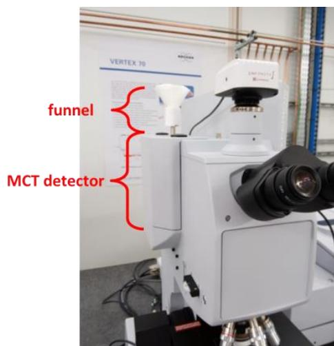
Figure 2: Detector filling with liquid nitrogen.
