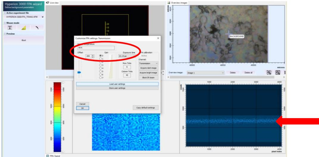
Click “Experts only” and set the next option “exposure time” and adjust the time in ms to bring a light blue line in the window and on the next image. Set OK and
