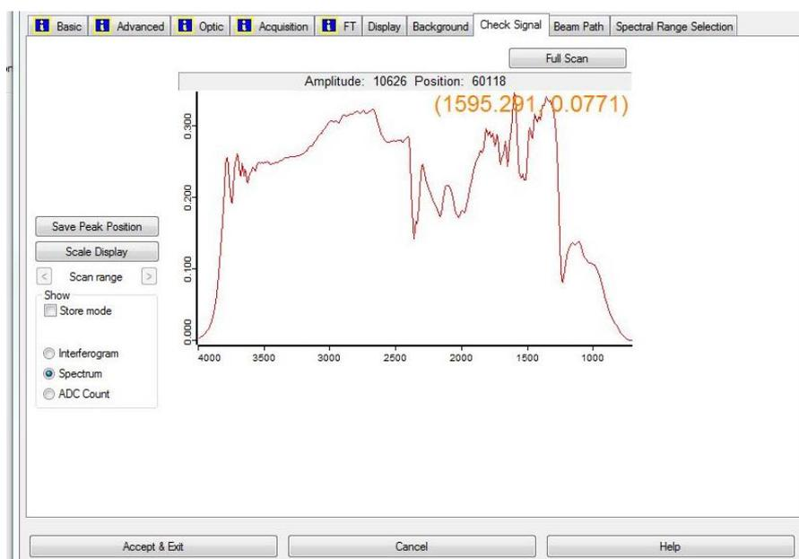
Tick spectrum to visualize the intensity and the Single beam spectrum shape. By aligning the condenser (only in transmission mode) and the mirrors of the matching box we aim to get the maximum amplitude and stability of the beam. (Note, if you are measuring using the internal source of radiation, then the matching unit is not needed for the alignment).
