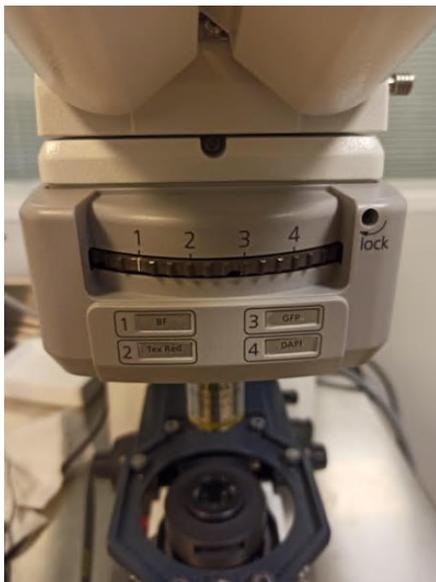
Emission filter wheel. Must click to be correctly placed.
