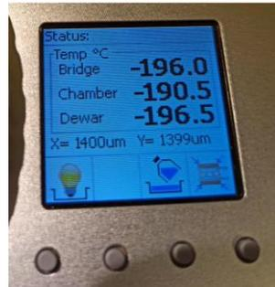
*Cryo-Linkam menu buttons: Left: cryochamber light on/off. 2nd: Bakeout start (only available when all LN2 is gone). 3rd: LN2 filling of cryochamber. 4th: rasters through the 3 sample positions. Pressed for 4s: access to menus for lid heater (normally on) and to LED for transmission measurements.*
