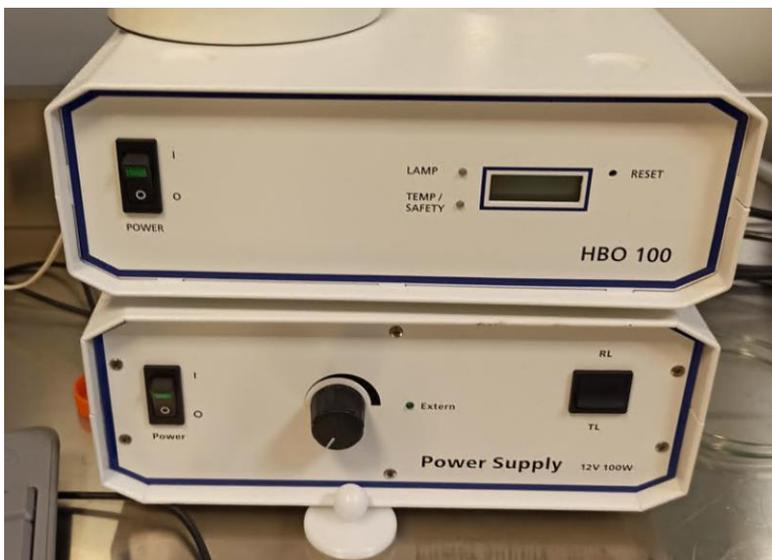
*Power supplies: upper for UV light, lower for visible/transmission (not usable with new Linkam stage, which has its own transmission LED).*
