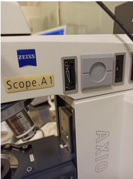
Top: UV light intensity wheel. Back slider at 1 to let UV light in. 2 = closed
