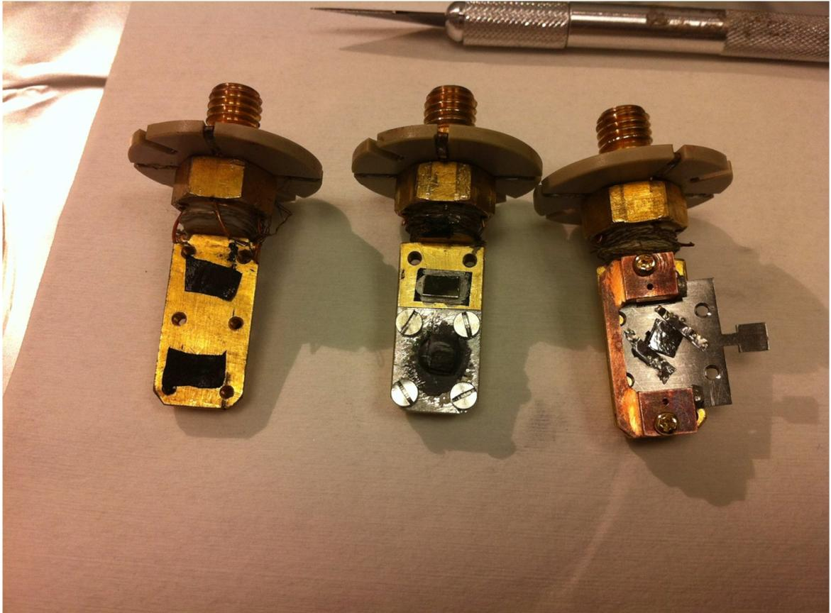
**Transmission setups. Membranes could be spot welded, silver paint stick (here below) or fixed with clips or plates, or others. Four contacts may be used or not as well, depending on sample mounting (i.e. if using an isolant plate stick ....)**
