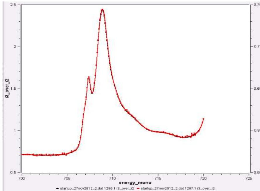
**Figure 1. BL29-BOREAS:** Comparison of two electron yield XAS measurements at the Fe L edge with (red line) and without (black line) the temperature stabilization feedback loop. The noise has been decreased by about a factor of 20, down to some 5 pico-Amps.
