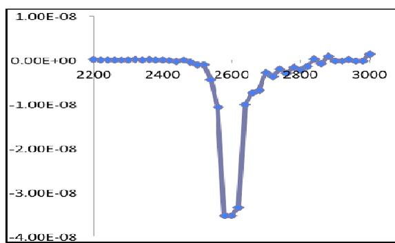
**Figure 1. BL11-NCD:** The differential photon beam intensity is shown as function of motor half-steps as one of the vertical slit blades in the guard slits is being moved through the beam. One half-step corresponds to a movement of  $0.5 \mu\text{m}$ . Signal was recorded with an ion chamber.
