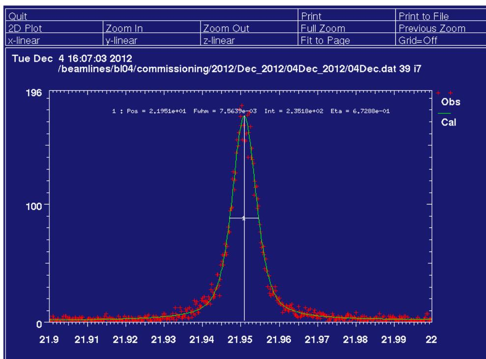
**Figure 1. BL04-MSPD:** The first measured Si 311 diffraction peak.
