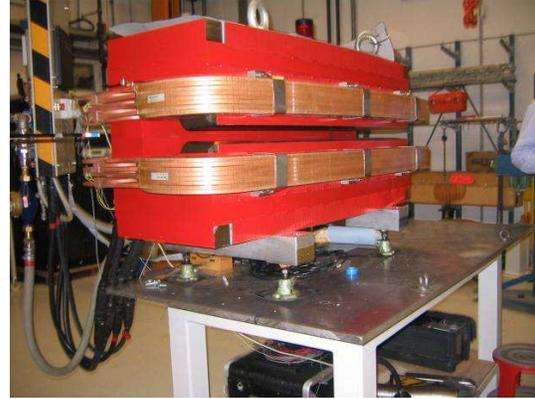
**Fig.9** Storage ring combined function magnet pre-series
