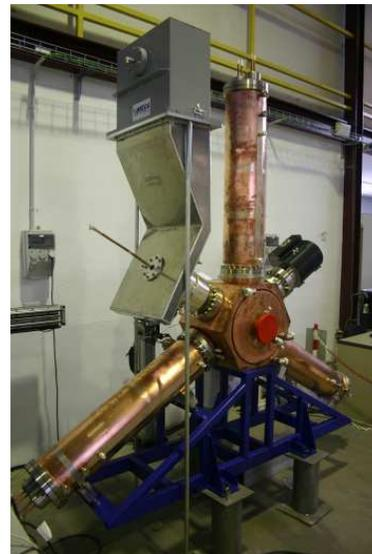
**Fig. 14** The prototype of the Dampy cavity and the Watrax for the storage ring.
