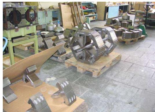
**Fig. 10** Quadrupole magnet for the storage ring and series of sextupoles being built at BINP in Novosibirsk
