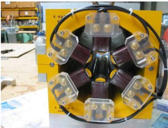
**Fig.11** Booster steering prototypes. Booster sextupole prototype
