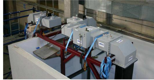
**Fig.13** Waveguide and load installed over the bunker in the RF lab.
