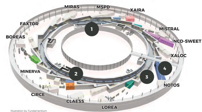
Booster ring: then the electrons are accelerated even further. now following a circular path, until almost reaching the speed of light.
