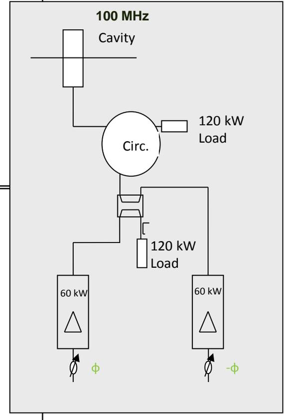
Alt I: Represents a solution for a 60% ID equipped ring, with the present MAX II/ MAX III cavities.
