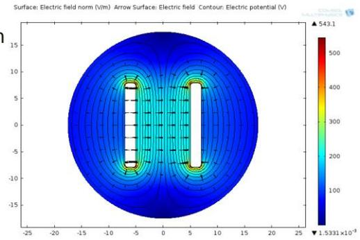
$$\begin{aligned} \text{If } \phi_1 = -\phi_2 &\rightarrow Z_0 = 49.9 \Omega \\ \text{If } \phi_1 = 0 &\rightarrow Z_0 = 63.8 \Omega \\ \text{If } \phi_1 = \phi_2 &\rightarrow Z_0 = 88.2 \Omega \end{aligned}$$
