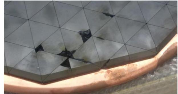
Ferrites are damaged severely.
