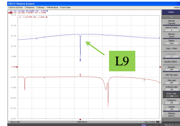
S22: signal from the antenna on the beam axis
