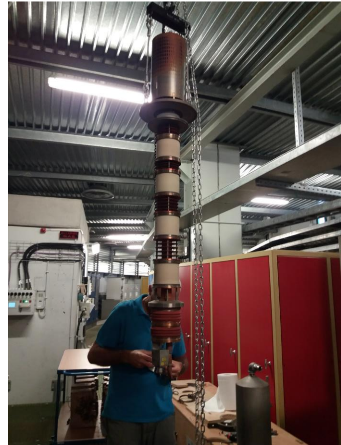
Philips YK1256 Klystron set into operation in 1991 in RF lab and then in RF# 3 in 2014, removed for low collector current after 42600.
