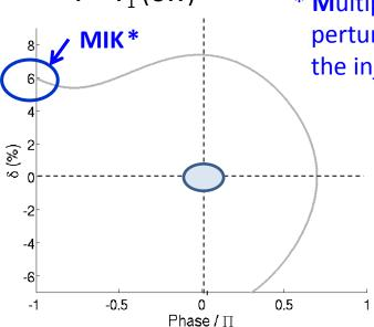
\* Multipole Injector Kicker  $\rightarrow$  Injection 6% off-momentum without perturbing the already stored beam; but with  $V_{RF} = 1.5$  MV only, the injected bunch would not be captured into the RF bucket.
