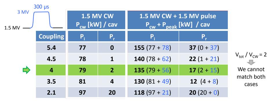
Incident and reflected powers ( $P_i$ ,  $P_r$ ) vs coupling factor assuming the use of 4 cavities ( $P_i = P_r + P_{dis} + P_{beam}$ ;  $P_{beam} = 65$  kW in all cases)
