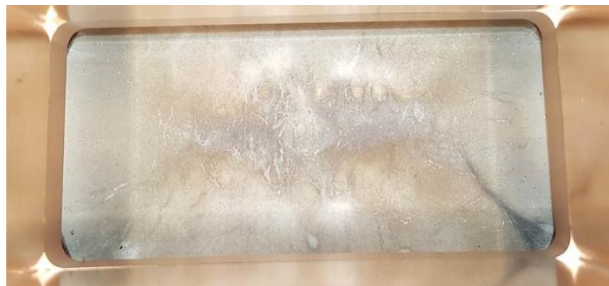
Damaged RF window in K02 – need to replace Klystron, rebake and recondition
