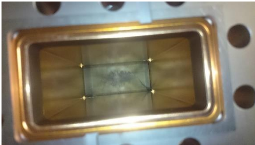
Damaged RF window in K02 – need to replace Klystron, rebake and recondition
