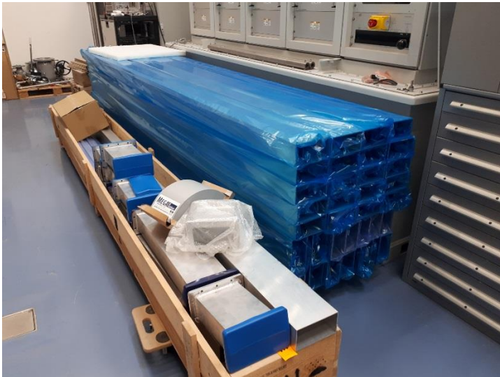
Waveguides, 20 kW circulator and 300 kW load
