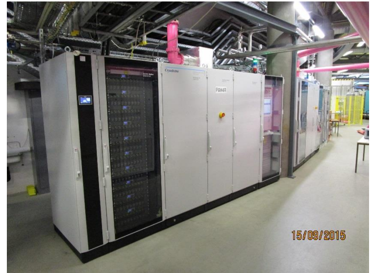
5-cell PETRA cavity installed in the booster and 80 kW 500 MHz SSA (from storage ring) by Cryoelectra
