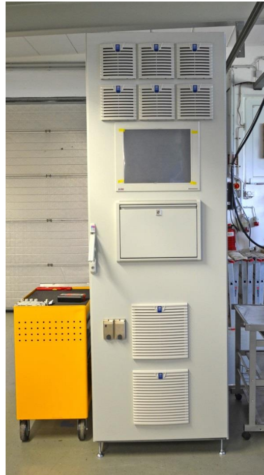
15 kW 1.3 GHz transmitter by Cryoelectra . Left picture front view and right side rear side door open. The power supplies in the upper part and the RF modules on the lower part of the rack. The waveguide is clearly seen.
