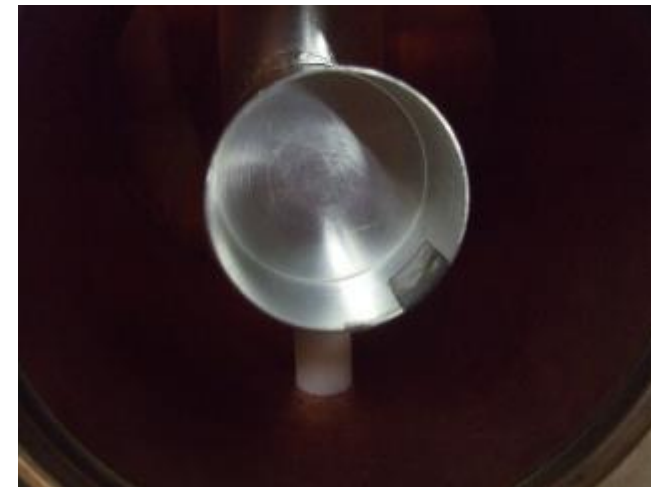
Bad contact from the inner clamp
