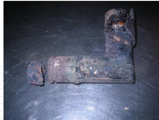
Inner elbow burned
