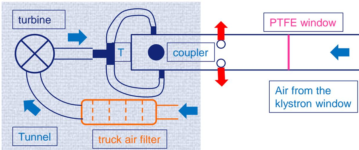
The air is taken in the tunnel, compressed with a turbine and blown on the coupler. It cools the waveguide including the coaxial line and escapes out of the tunnel.
