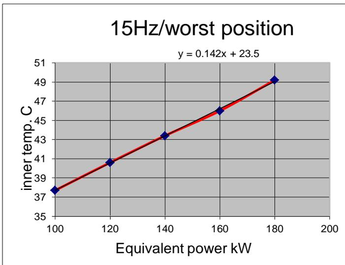
With an equivalent power of 283 kW, the temperature would not rise above an acceptable 64°.
