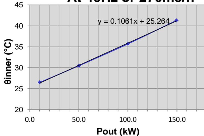
There is a linear dependency between the temperature of the inner conductor and the power.
