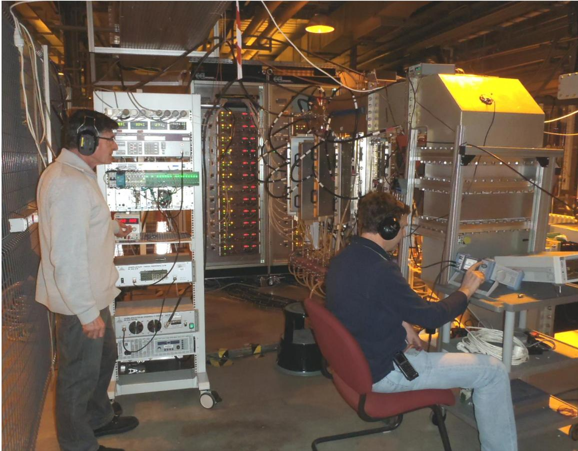
Reminder: we designed and built an RF amplifier at 352 MHz based on a cavity combiner (see CWRF presentation).
