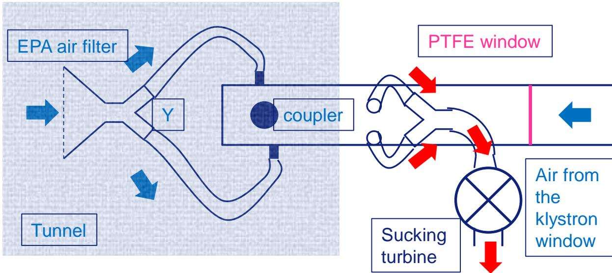
The air is taken from the tunnel, divided with a Y and blown on the coupler insulator. It cools the waveguide including the coaxial line, is sucked by a turbine outside the tunnel
