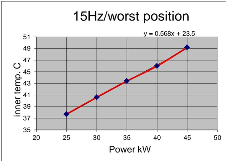
As the temperature probe could not be moved, the temperature depends on the short-circuit setting.
