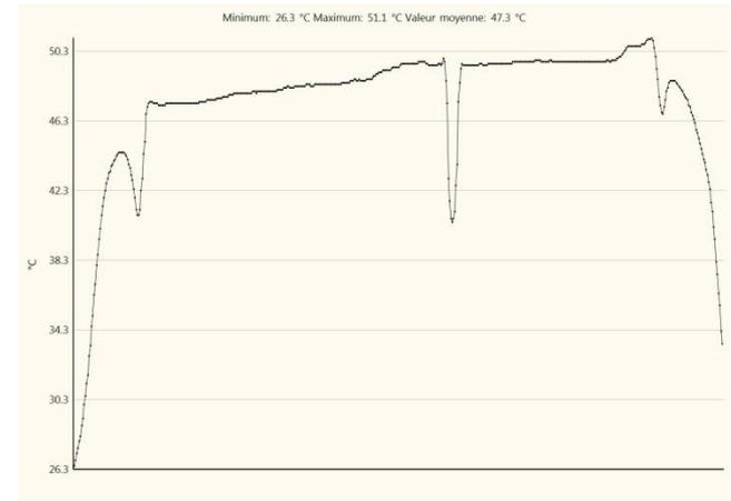
Temperature distribution measured with IR camera and optic fiber probes
