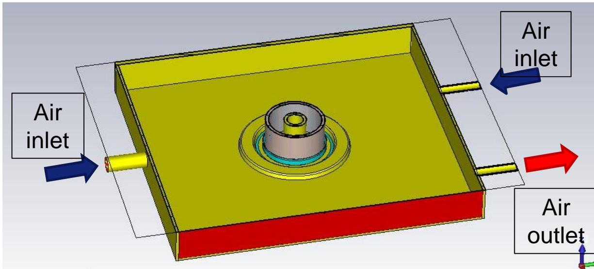
The air is taken in the tunnel, filtered with a truck filter, compressed with an ELMO-RIETSCHLE turbine, divided with a T and blown on the coupler insulator. The exhaust is in the tunnel. The pressure drop is high, due to the small diameter of the inlet and outlet pipes (26mm ID).
