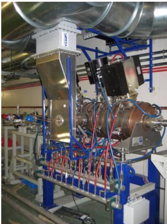
Tunnel: 5Cell Cavity – 500MHz
