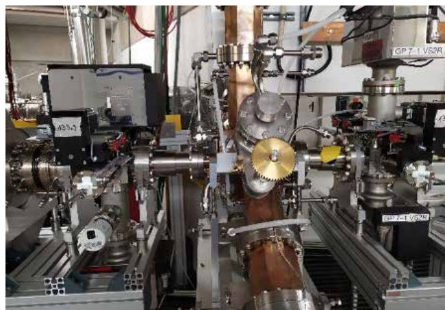
Figure 4-13: 3 rd harmonic cavity installed in the Bessy II ring for the performance tests.
