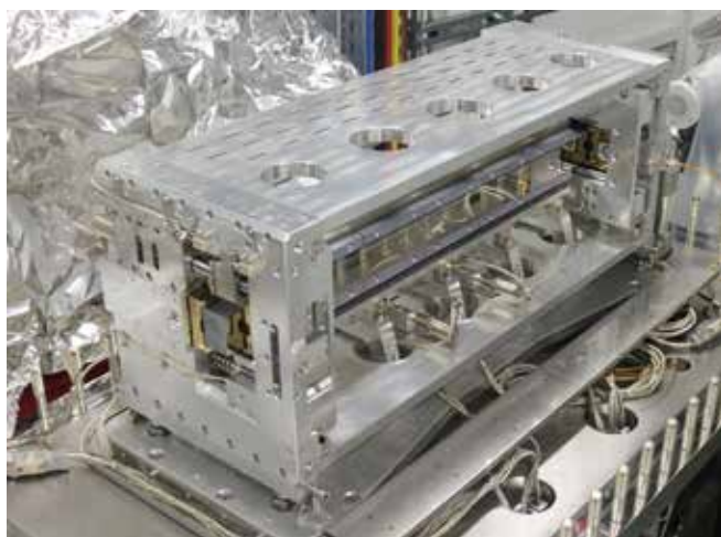
Figure 5-3: Example of adaptive optics system installed at the XAIRA beamline at ALBA. It includes two bending actuators and two adaptive correctors, used to correct the thermal bump. The system includes also the water cooling of the mirror.
