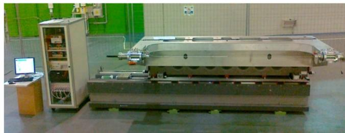
**Figure 1:** Design and picture of the new Hall probe bench prototype built at CELLS.
